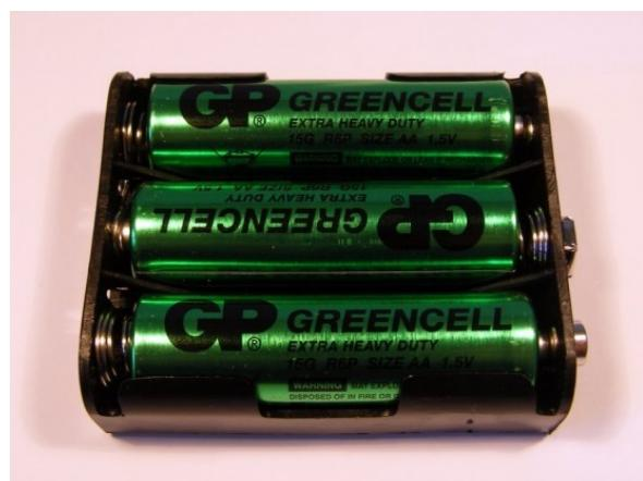
11. You can now attach the board to the battery box using an elastic band - we suggest you use the bottom (plastic) side of the battery box as sometimes the bottom of the circuit can be sharp, cutting through the paint on the batteries and causing short circuits.
