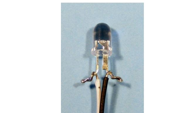
7. Cut the length of heatshrink tubing into five pieces. Heatshrink was not provided in 2010 edition kits - you can use sticky tape instead. Place a piece over the negative (black) wire of each LED and push right up against the LED. Shrink the tubing by holding it as near to the soldering iron as you can without touching it - about half an inch up from the tip works best. If you do touch the heatshrink with the iron, wipe off any molten plastic as soon as possible on the brass tip cleaner.
